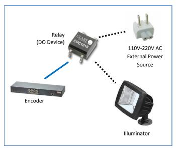
The illustration below is a graphic example of connecting a relay to a high voltage DO device.
